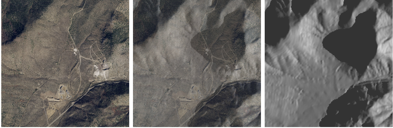
Figure 4.1: Orthoimagery of an area near Eureka, UT (left), the calculated lighting map overlaid on the orthoimagery (middle), and the lighting map L(z, \mathcal{P}) (right). This was one of the areas we used to test flight paths planned using the VTTP metric. The lighting map was computed for 8:20 a.m. on Sep. 15, 2011, with A = 0.2 .
